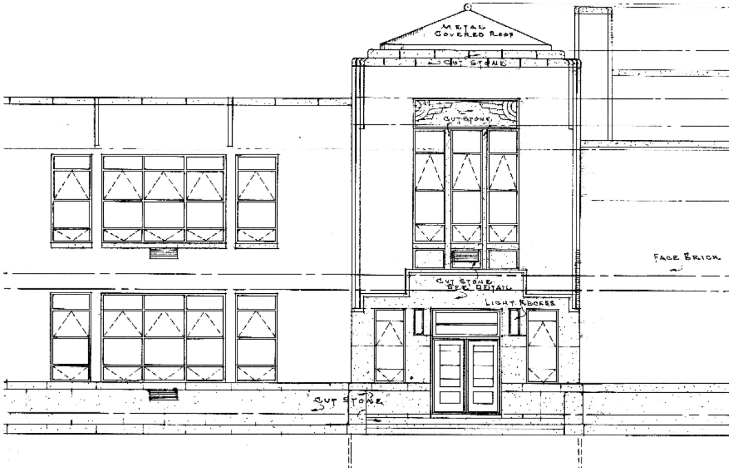
Figure 6. Detail of the east elevation, showing the hipped roof of the entry tower as designed. Source: Ralph Scamell, May 1937, Sheet 6.
